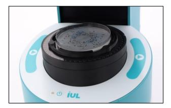
After pushing the button, the diffusing sphere (2) will descend to cover the Petri dish, the lighting and image acquisition procedures will be performed, and finally, the diffusing sphere will return to its upper resting position. Then the process results will be displayed on the screen.
