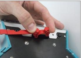
Once extracted, save the securing device to re-use it in future shipments, since it is essential for the safe transport of the SphereFlash®.
